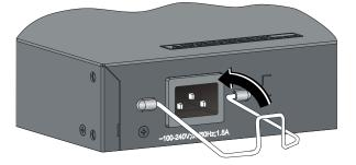
Figure 3-16 Connect an AC power cord to a horizontal AC power socket (2)
